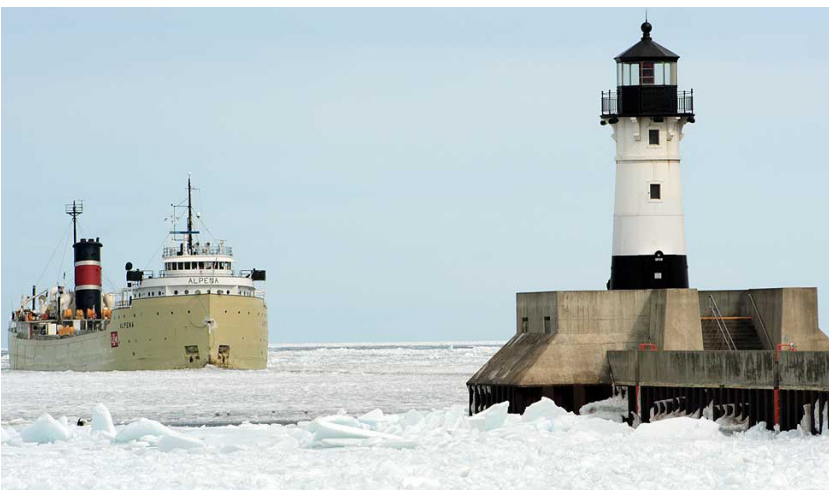
The cement carrier ALPENA (left) marked its 70th year of operation in 2012. Launched in 1942 as the ore carrier LEON FRASER, the ship was converted to haul cement in 1991. The Lakes' freshwater environment means a well-maintained hull can last almost indefinitely and, with adequate Coast Guard icebreaking resources, operate from early March until mid-January. Photo courtesy Travis Chadwick.
