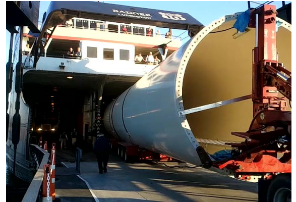
It's been a long time since the car ferry BADGER carried railroad cars, the cargo for which she was built, but now her cavernous hull is ideally suited for wind turbine parts. Photo courtesy Lake Michigan Carferry Service.
