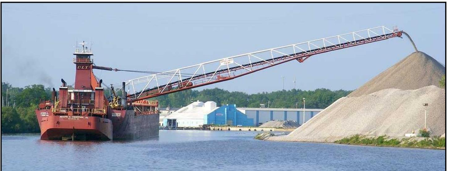
Positioning the unloading boom as close as possible to the receiving stockpile is again the industry standard as it is important that there be as little breakage as possible. This is particularly true for iron ore pellets.
